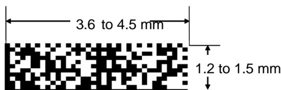
(2) When approx. 3 mm square of marking area cannot be assured on the steel instrument due to its rod shape
