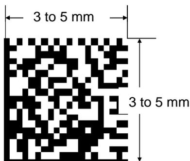
(1) When 3 mm or more square of marking area is assured on the steel instrument
